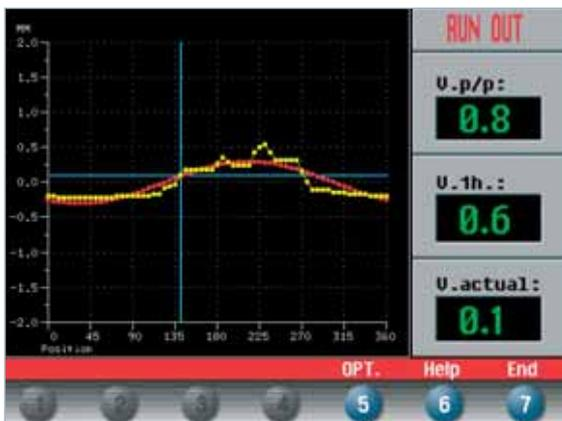
EMS eccentricity measuring system (1st Harmonic and Peak to Peak) through Sonar (option). It is automatically activated during balancing cycle allowing operators to get the information about wheel eccentricity without any time loss.
