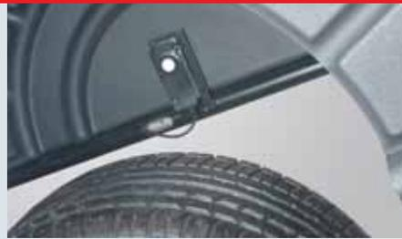
LA optional automatic wheel width measure using the SONAR system (CEMB patent), with no operator manual intervention.
