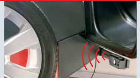
EMS optional no contact measurement system of wheel radial eccentricity through SONAR during balancing cycle (CEMB patent).
