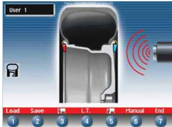
LA automatic wheel width measurement through CEMB patented sonar system (option).
