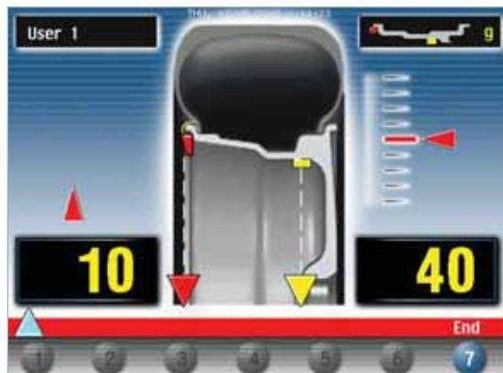
ALU-S function with "intelligent" gauge (automatic input of diameter and distance rim/machine) for correction on two planes inside of the wheel. Axial weight position indication for wheel in ALU-S and correction in a hidden position.
