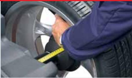
The correction planes set inside the wheel, can be found with distance gauge after the measure spin. A handy pincer allows the counterweight application in the exact correct position.
