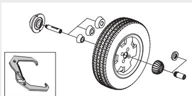
► **UC20-SE2 cone adaptor** for wheels with central hole  $\varnothing$  from 43 to 110 mm.
