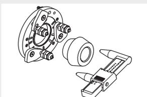
► **UH20/2** for wheels with 3-4-5 holes, with/without central hole on a  $\varnothing$  from 95 to 210 mm. The additional cone (CEMB patent), in the majority of cases, allows to center the wheel from inside on the central hub seat, thus improving balancing accuracy respect to the traditional adapters on the market.
