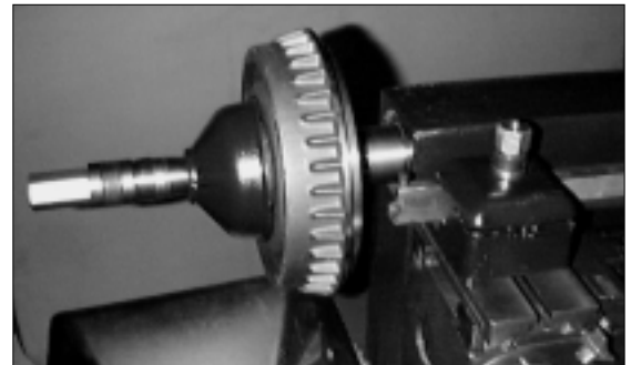
Figure 7 - Drum and Boring Bar Mounted on Lathe
