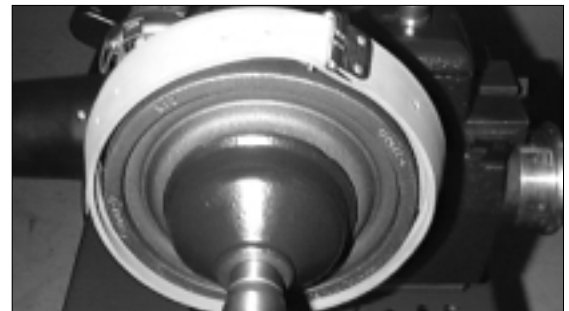
Figure 8 - Wrap Silencer Band Around the Drum
