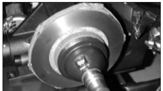
Figure 17 - Attach Silencer Band
