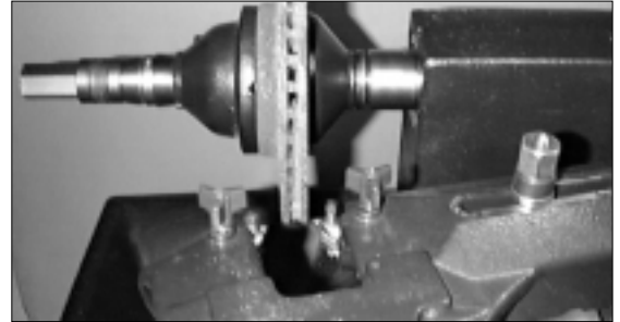
Figure 14 - Mounted Rotor and Initial Twin Cutter Position
