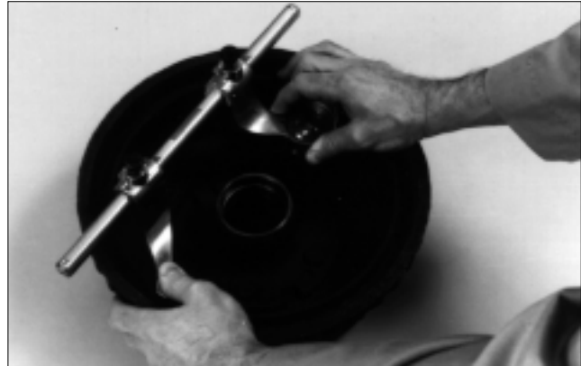
Figure 5 - Measure Drum Diameter
