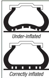
under-inflation. However, under-inflation can cause many tire-related problems. As inflation pressure largely determines a tire's load capacity, under-inflation results in an overloaded tire. An under-inflated tire operates at high deflection resulting in decreased fuel economy, sluggish handling and may result in excessive mechanical flexing and heat build up, leading to catastrophic tire failure.
