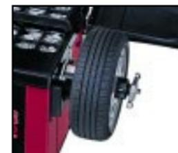
Coats continually studies the balancing process. This helps shops who use our equipment provide the best balancing accuracy for their customers. We enhance the performance of our balancers with accessories that ensure correct clamping and mounting of wheels. Improper mounting is the overwhelming cause of balancing errors.
