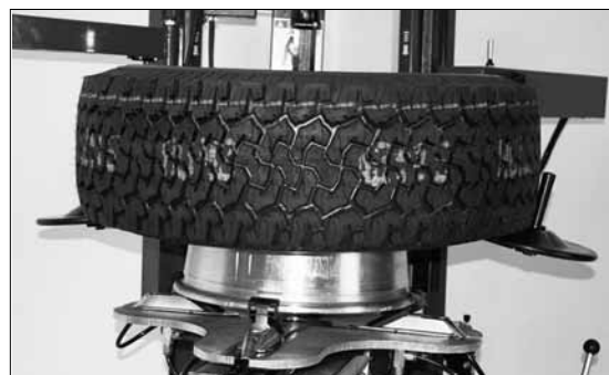
Figure 12 - Lift the Tire for Lower Bead Removal
