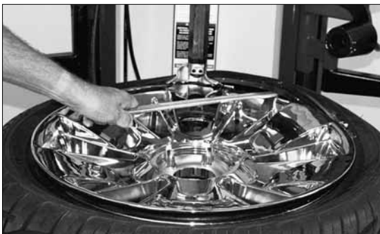
Figure 35 - Start Upper Bead Removal
