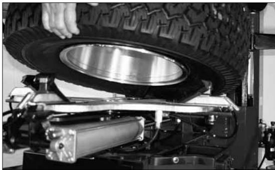
Figure 5 - Clamp Outside on Mag Wheels
