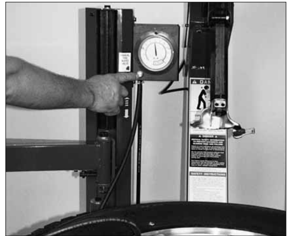
Figure 22 - Location of Manual Release Valve
