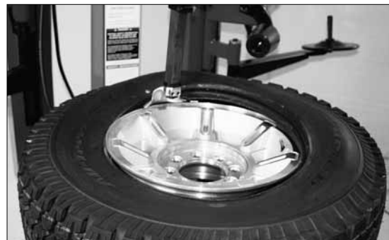
Figure 11 - Demount Upper Bead
