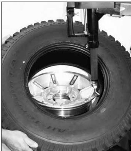
Figure 17 - Position Tire Against Duckhead
