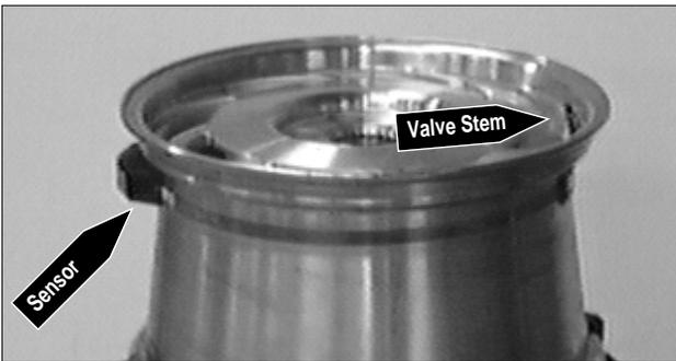
Figure 23 - Wheel with Low Pressure Sensor/Transmitter
