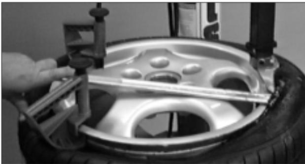
Figure 29 - Pull Lifting Tool Down and Rotate Wheel
