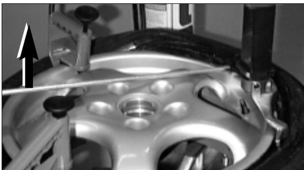
Figure 35 - Use Hooked End of Bead Lifting Tool
