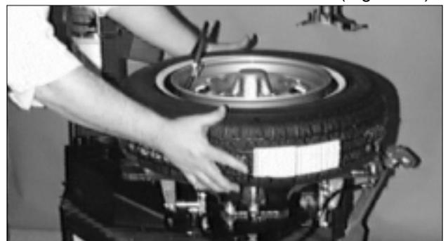
Figure 17 - Lift Tire Upwards for Bead Sealing
