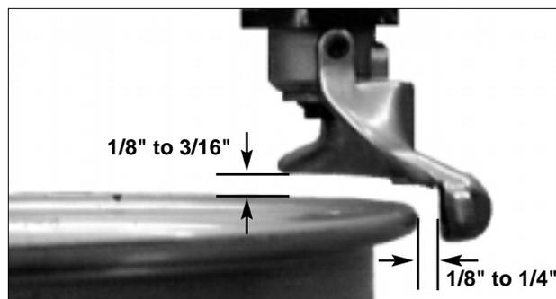
between the top of the rim edge and the bottom of the head, and 1/8 to 1/4 inch clearance between the rim edge and the head roller. This clearance will be maintained as long as the locking handle and adjustment knob are not changed. The operator may swing the arm out of the way and back into place again without needing to reposition the head (when changing a like set of wheels) (Figure 8).
