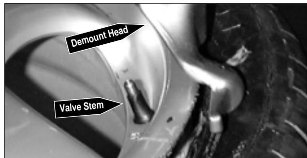
Figure 27 - Position Valve Stem Under Demount Head
