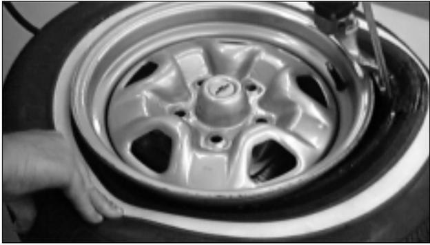
hand to press down on the tire opposite the head to help with tool insertion (Figure 9).
