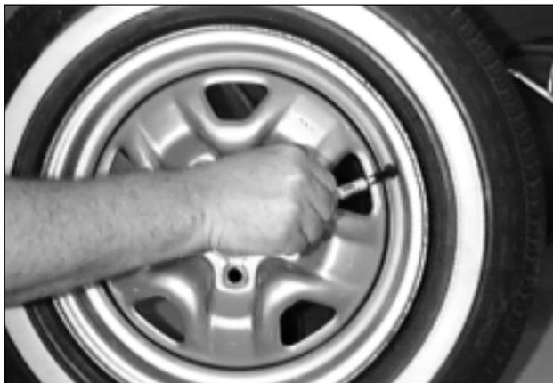
Figure 1 – Remove Valve Core to Deflate Tire
