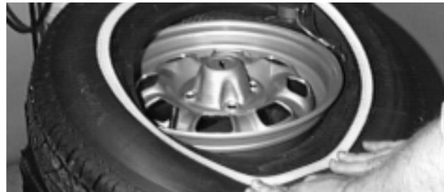
Figure 16 - Mounting Top Bead
