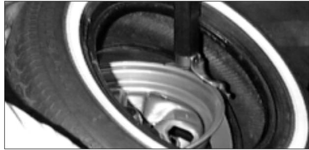
Figure 15 - Position Tire Against Mount/Demount Head
