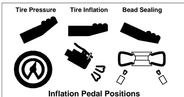
**Position 1 - Tire Pressure** – With the inflation hose attached to the tire valve and the pedal in this position, the air gauge will register the air pressure in the tire. Whenever your foot is removed from the pedal, it will return to this position.
