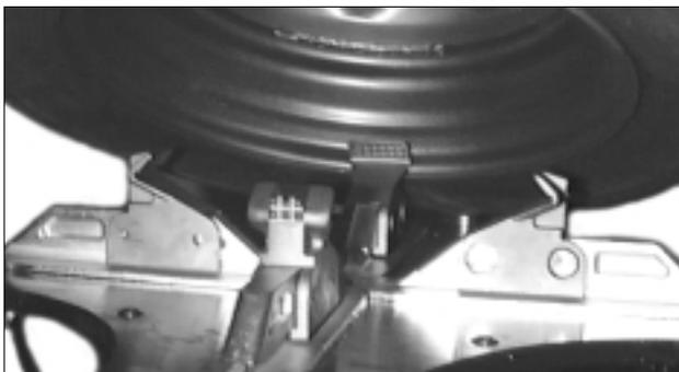
Clamp steel wheels from the inside (clamps push outwards against wheel). Clamp mag and custom wheels from the outside (clamps push inwards against the outside rim edge). Refer to the Performance Tires and Wheels section.
