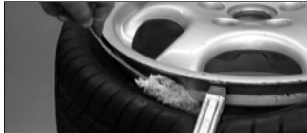
Figure 26 - Lubricate Upper Bead
