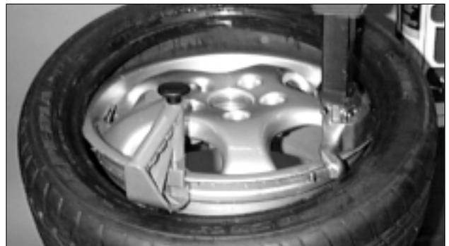
Figure 33 - Mounting Top Bead
