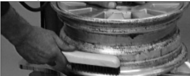
Figure 13 - Inspect and Clean the Wheel
