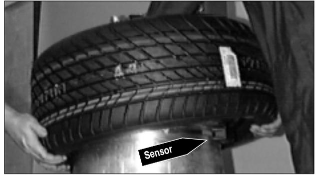
Figure 31 - Use Help on Lower Bead, Watch Sensor
