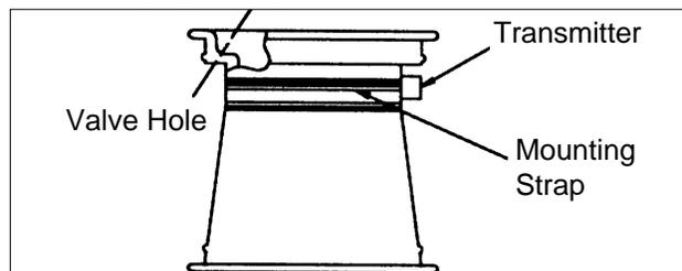
Figure 38 - Wheels with Low Pressure Sensor
