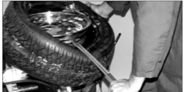
Figure 32 - Mount Upper Bead, Use Lifting Tool
