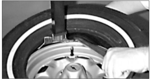
smooth curved end of the bead lifting tool down over the forward end of the mount/demount tool and below the lower bead. Lift the bead up and over the knob on the demount head (Figure 12).
