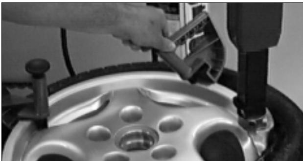
Figure 30 - Remove Drop Center Tools Before Tool Head
